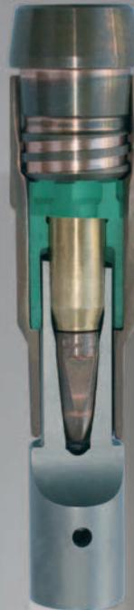
**ICS (Integrated Cleaning System).** This system enables the complete elimination of spatter build-up on weldings prone to spatter. Protected and easy-to-clean fastening and gas vent systems. High-level of refrigeration reducing gas consumption. Auto-adjustable length of milling entry point.
